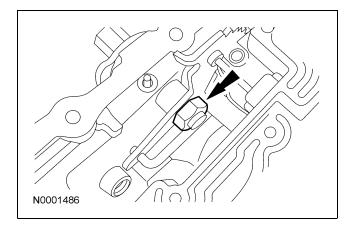
14. CAUTION: The tabs on the output shaft thrust washer (No. 11) point into the case. Make sure the thrust washer is correctly seated.
